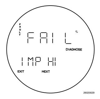
Figure 6-10. Fault 6, Cell Impedance Too High
